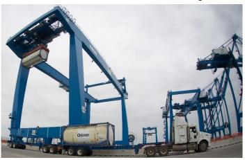
Figure 2 External trucks at the ASC stack
