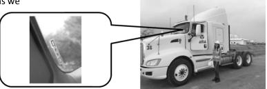
Figure 6 Windscreen tag fitted to the truck
