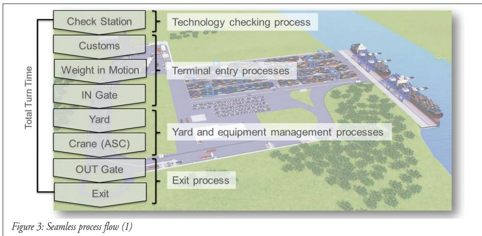
Figure 3: Seamless process flow (1)
