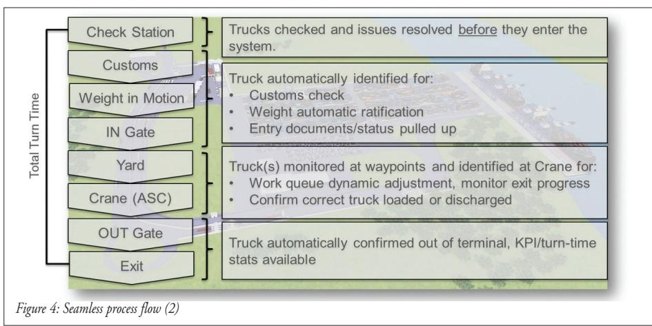
Figure 4: Seamless process flow (2)
