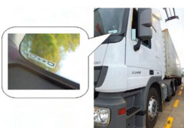
Figure 1: Low cost tag used for external trucks
