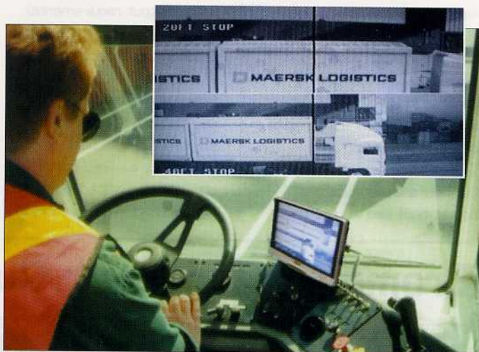
■ Typical in-cab arrangement. (Inset): Typical split screen view for a 20' and 40'/45' foot container
