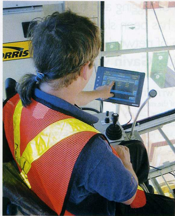
Twistlock override functions prevent RTG drivers doing wrong moves or picking the wrong boxes
