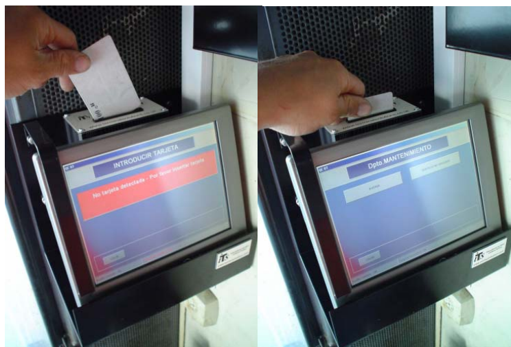
Touch screen VMT complete with card access system. RDS connection to security & maintenance server
