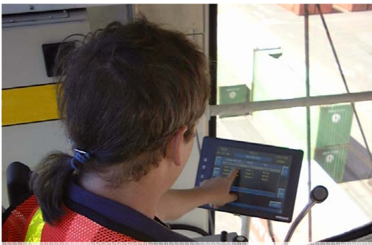
Yard equipment operator using ITS touch screen RDS. The system is integrated to a fully automatic PDS system
