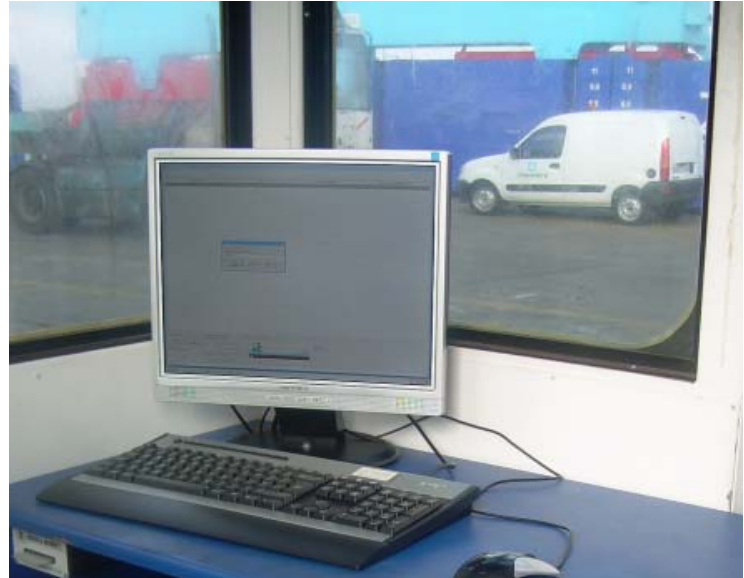
Standard Low cost PC installed in STS checkers cabin connected to an ITS RDS for ship load and discharge
