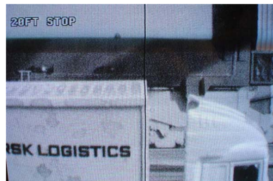
Typical drivers view of the 20' screen with the load being positioned on the corner castings.
