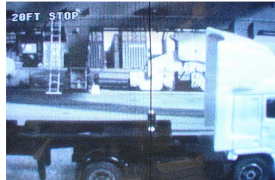
Typical drivers view of the 20' screen with the chassis positioning on the twistlocks.
