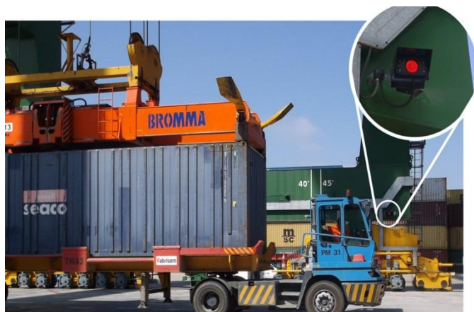
Figure 1 Prime Mover Stopped in the Correct location
