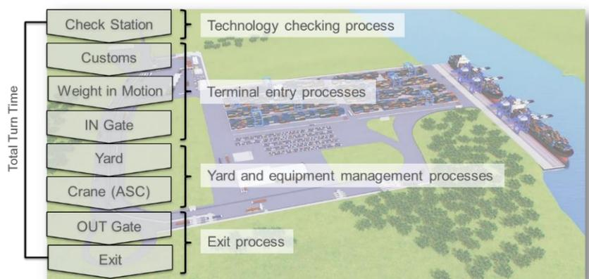
Figure 3 Seamless process flow (1)
