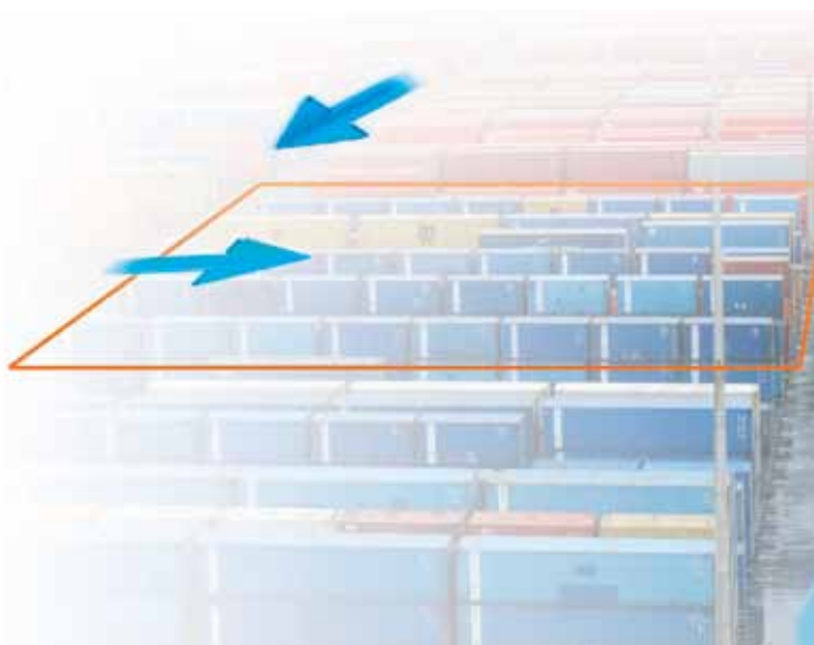
'Geo Fences', which sub-divide the terminal into a number of Job Steps.
