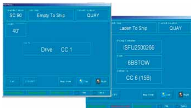
Sample initial Job Step Screen for a Straddle Carrier. The screen automatically changes when a Geo-Fence is passed.
