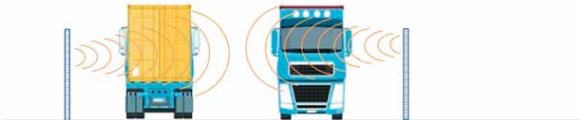
Portals at each ASC Lane to detect Truck ID and direction.
