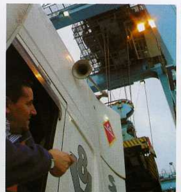
The truck driver points the unit at the RTG. The RTG automatically identifies truck, container and planned yard location
