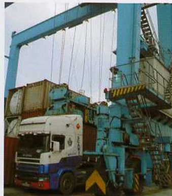
In the yard – a container move instruction is sent to the RTG as the truck driver travels to the designated yard location
